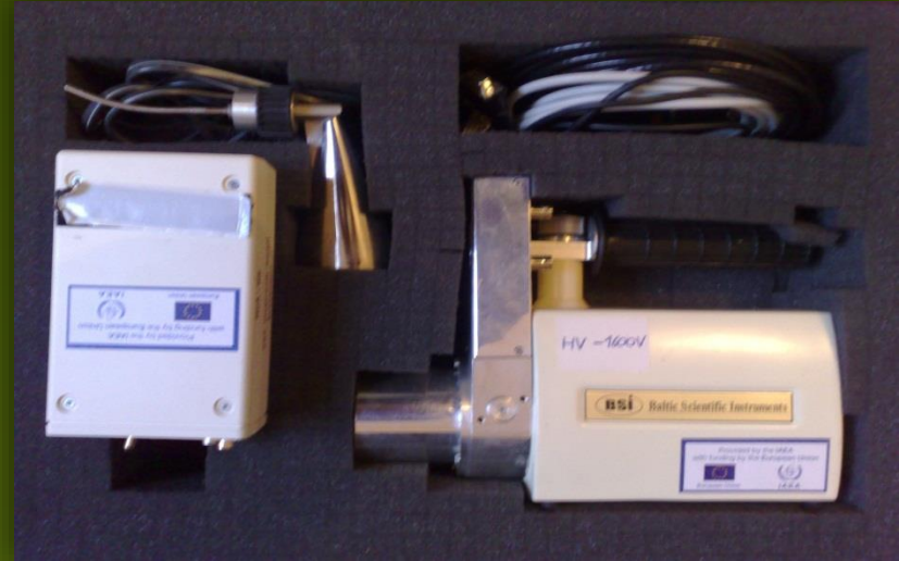
HP Ge handheld Spectrometr, BSI
