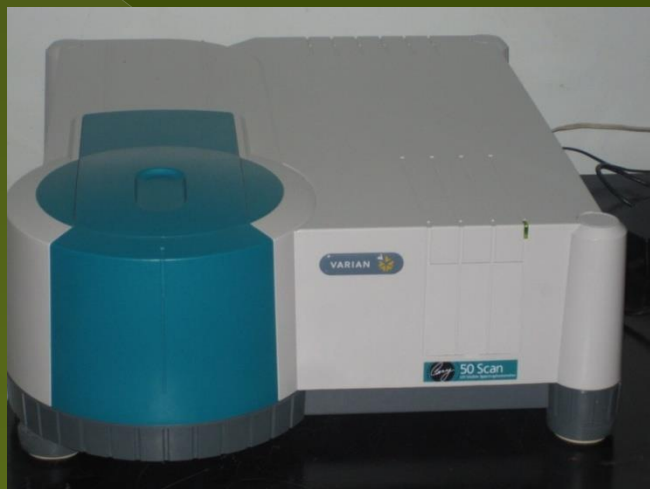
UV-Spectrophotometer, Varian (200-800nm)
